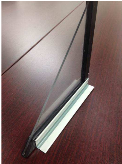
Figure A2 – Window Insulators Panel Magnetized to Steel Angle
