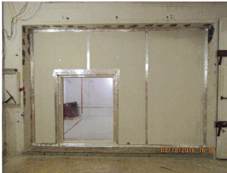
Figure 2. 1418 mm high x 1138 mm wide single pane wood window was mounted in the 2440 mm high x 3658 mm wide filler wall.
